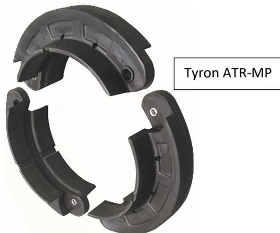
The TYRON patented modular Rubber All-Terrain modular systems are designed to be fitted and removed with standard workshop tools in the field. Not only do they make large, heavy, and expensive hydraulic machines obsolete, they significantly reduce the costs of logistics mentioned above, and the significantly reduced vehicle down time means the soldier remains best supported and protected.
