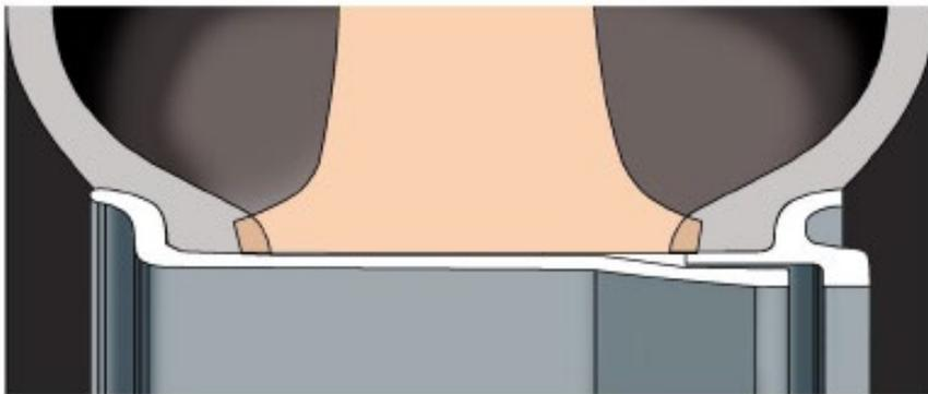
Rubber runflats are over manufactured in width to allow for the manufacturing tolerances of the wheels and tyres, ensuring tyre bead compression during the installation, guaranteeing the beadlock, as you can see in the above illustration.
