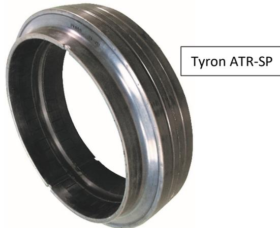
The one-piece system, common in many markets around the world, requires a large hydraulic press to insert or remove the runflat from the assembly when changing tyres. This requires the wheel & tyre assembly, or indeed the whole vehicle to be taken to a base with the appropriate equipment on site, or in many cases, the logistical challenges, and costs of freighting the assemblies to a third-party base or even another country.
