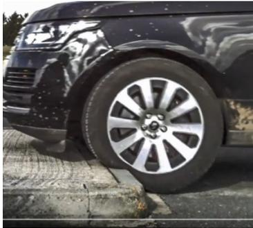
Rubber will absorb shock from impingement caused by curb strikes, potholes and operating in generally hostile environments. Rubber drastically reduces the vibration and stresses that are transmitted through the runflat to the wheels, axles and drive shafts allowing you to continue with little change to the handling of the vehicle whilst retaining a degree of comfort for the driver and passengers.
